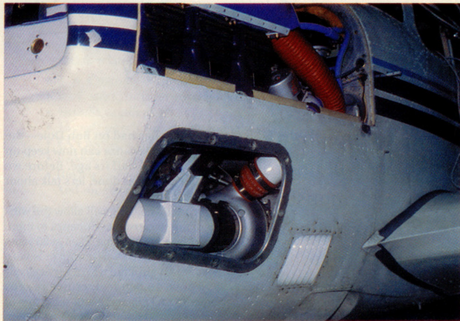
Looking through the lower left engine access panel, the silver scroll of the compressor side of the turbocharger can be seen. Filtered inlet air is delivered to the turbo via ducting from the front of the engine compartment. The compressed-air ductwork can be seen exiting the top of the scroll.
